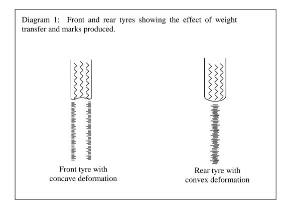
The track between the front and rear sets of marks can be measured and if the final resting point can be identified, the wheelbase can also be measured. In accidents where a vehicle has failed to stop, this can provide important information about the missing vehicle.
