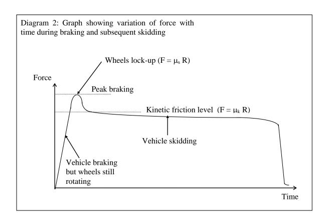
There is a sharp rise to maximum braking as the driver applies the brakes. As the wheel locks the force produced drops slightly and is followed by a lengthy period where the force produced is more or less constant. This corresponds to the time while the vehicle is skidding. The vehicle therefore slows at a roughly constant rate, until it comes to a halt.
